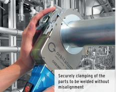
The small dimensions of the ORBIWELD "S" series make it ideal for applications where space is very restricted, such as the pharmaceutical and chemical industry, the semiconductor, food and beverage industry as well as aerospace.
